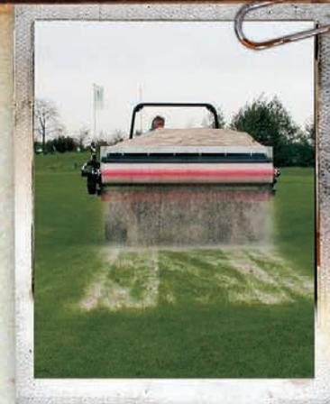
The 12 series top dressers offer you the widest brush applicator top dresser available with a smooth even spread, over 6 ft. wide. This makes the 1210 body mount spreader ideal for fitting onto your utility vehicle, as its spreading width will be outside the vehicle's wheel width. The 1210 is a trailed unit for use behind any prime mover.
