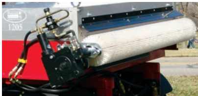
Delivery and metering system
