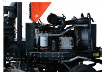
50.2 HP (37.4 kW) diesel Kubota® engine
