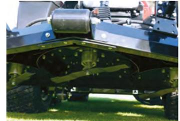
Low maintenance, direct drive hydraulic decks
