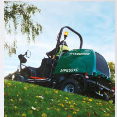
Tilt sensor technology warns of unsafe working angle
